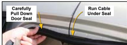
For a more professional looking installation, run the antenna cable under the door seal. Carefully pull down the door seal. Run the cable under the seal and push the seal back into place. This prevents constant wear and tear on the cable as the door opens and closes. The antenna cable is small enough to easily tuck under the door seal or plastic molding.
