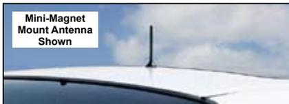
The Outside Antenna must be installed vertically. Antenna performance will be degraded if the antenna is not vertical.
