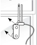
Attach the suction cup bracket to the inside of a window so that the cable will reach the location of the Sleek. Place the bracket as high on the window as possible for best performance.
