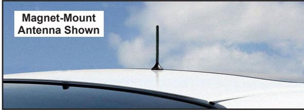
The outside antenna must be installed vertically. Signal performance will be degraded if the antenna is not vertical.
