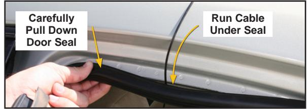
For a more professional-looking installation, the antenna cable may be run under the door seal. Carefully pull down the door seal. Run the cable under the seal and push the seal back into place. This prevents constant wear and tear on the cable as the door opens and closes. The antenna cable is small enough to easily tuck under the door seal or plastic molding.
