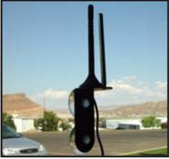
Once the bracket is in place, attach the magnet base of the antenna to the flat surface of the bracket. Note: the antenna must be installed vertically. Signal performance will be degraded if the antenna is not vertical. The antenna cable is small enough to easily tuck under the door seal or plastic molding.
