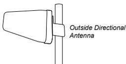
Place the inside antenna directly beneath the placement of the Outside Antenna location
