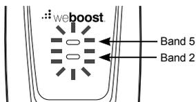
**Green** indicates that the booster is powered and operating at maximum gain.
